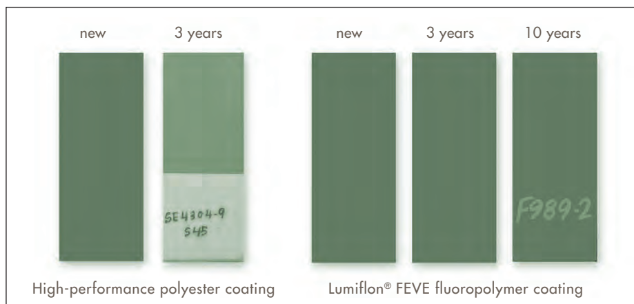
FIGURE 1: COMPARISON OF DURABILITY BETWEEN HIGH-PERFORMANCE POLYESTER AND LUMIFLON® FEVE FLUOROPOLYMER COATINGS
